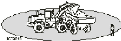
The danger area around an operating machine forms a circle with a radius of least 7 m (23 ft).
